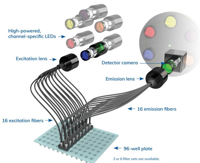
Figure 1. Innovative Cielo Real-Time PCR system optics.
